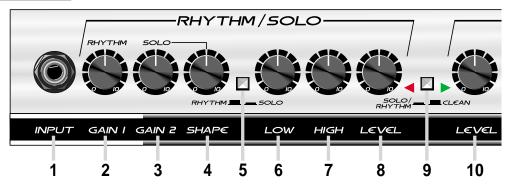
1: INPUT: Use this 1/4" jack to connect your guitar to the amplifier by means of a shielded instrument cable.
